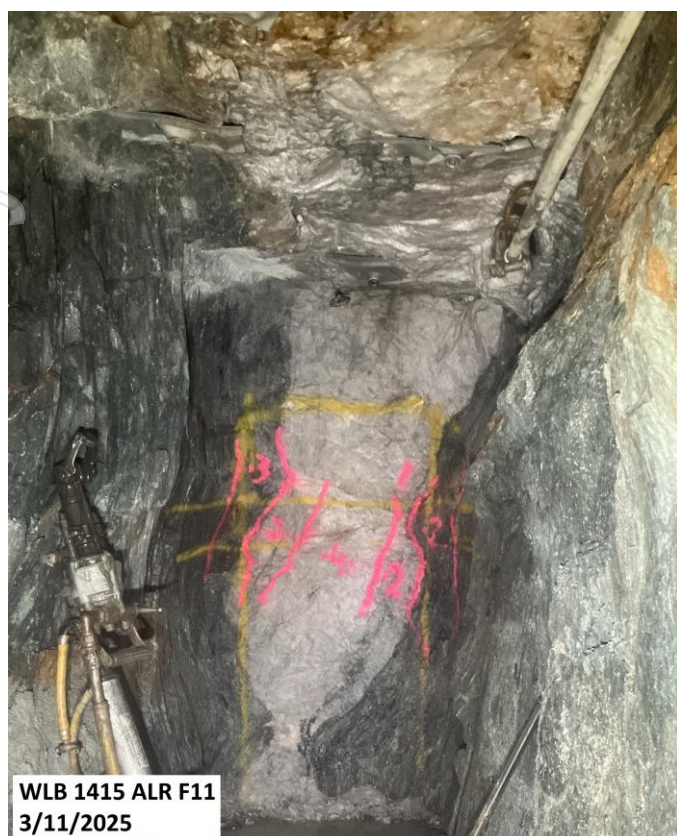
Figure 11: Airleg development face photo from face #11 on 1415 level (average face grade: 1.3m @ 29.5g/t Au, inc. 0.6m @ 58.8g/t Au ).
