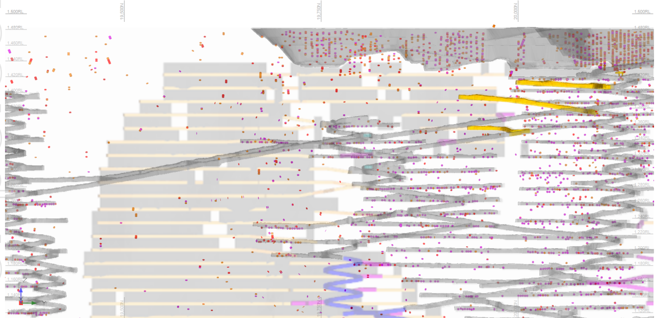
Figure 6: Long section showing focus area for FY26 ore development (within ~200m of surface), current development on the Wilber lode (yellow), planned stoping and development (transparent), previously reported drilling results and face sample grades from previous ore drive development.
