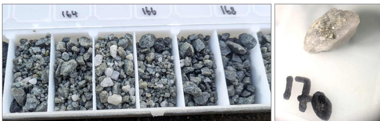
Figure 3. RC chips from SJRC003, highlighting a zone of strong sulphide alteration and quartz veining.
