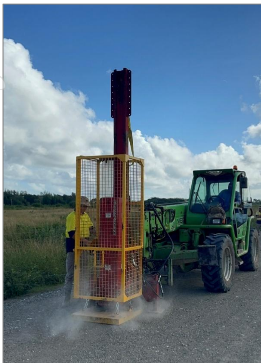
Figure 4 – “Thumper” weight-drop system in action
