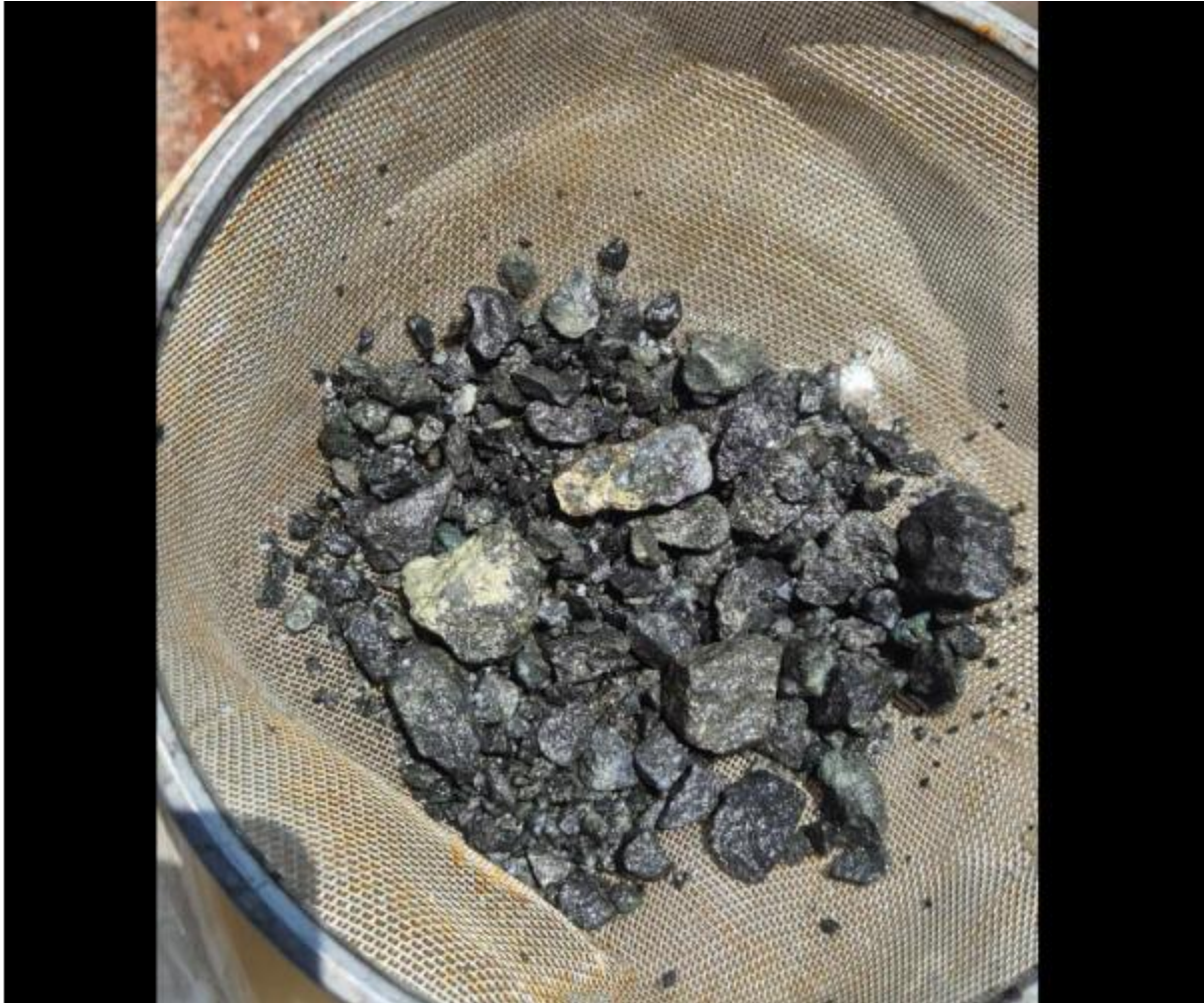
Figure 2 - Image showing dominantly finely disseminated and minor semi-massive Cu-Zn mineralisation within strong, pervasive calc-silicate alteration (olivine, pyroxene, amphibole, relict marble), 149-150m, OGRC010. Visual estimates ~7% chalcopyrite (2.3% Copper) and ~4% Sphalerite (2.7% Zinc). Note: Visual estimates of mineral abundance results should never be considered a proxy or substitute for laboratory analyses where concentrations of grades are the factors of principal economic interest. Visual estimates also potentially provide no information regarding impurities or deleterious physical properties relevant to valuation
