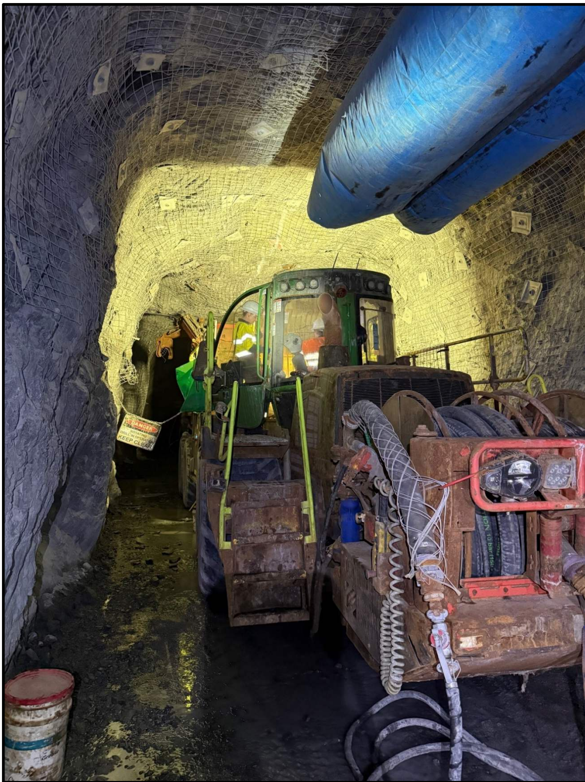
Figure 10: Barminto Rhino Rig drilling a boxhole in the first stope to be mined at Dalgaranga
