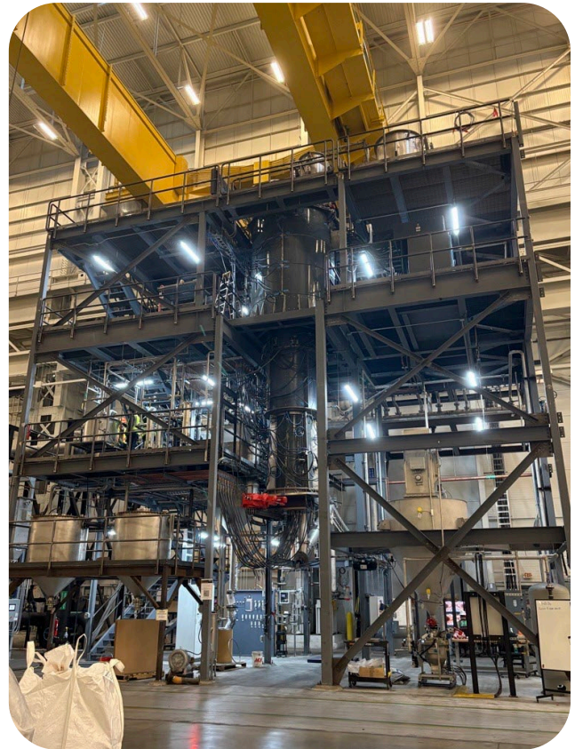
Figure 1 Mass Production Furnace at Riverside Facility in Chattanooga, Tennessee.
