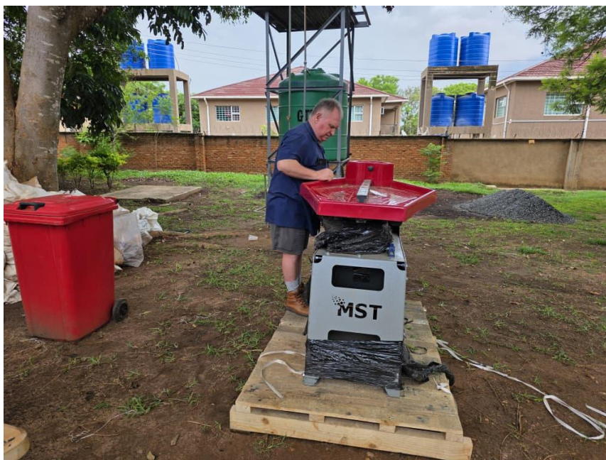
Figure 4. Senior Geologist Leon de Waal inspecting one of the two new Gemini wet shaking tables used for gravity separation during sample processing.
