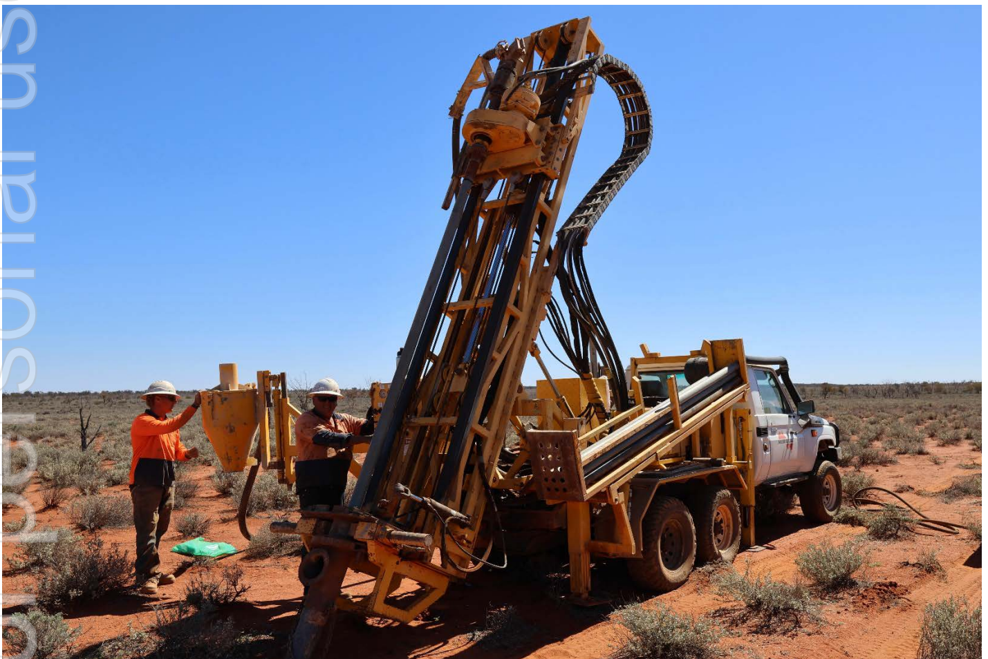
Figure 4: Landcruiser mounted AC Drilling underway at Ariadne-Company Well prospect areas, Minos Gold Project.
