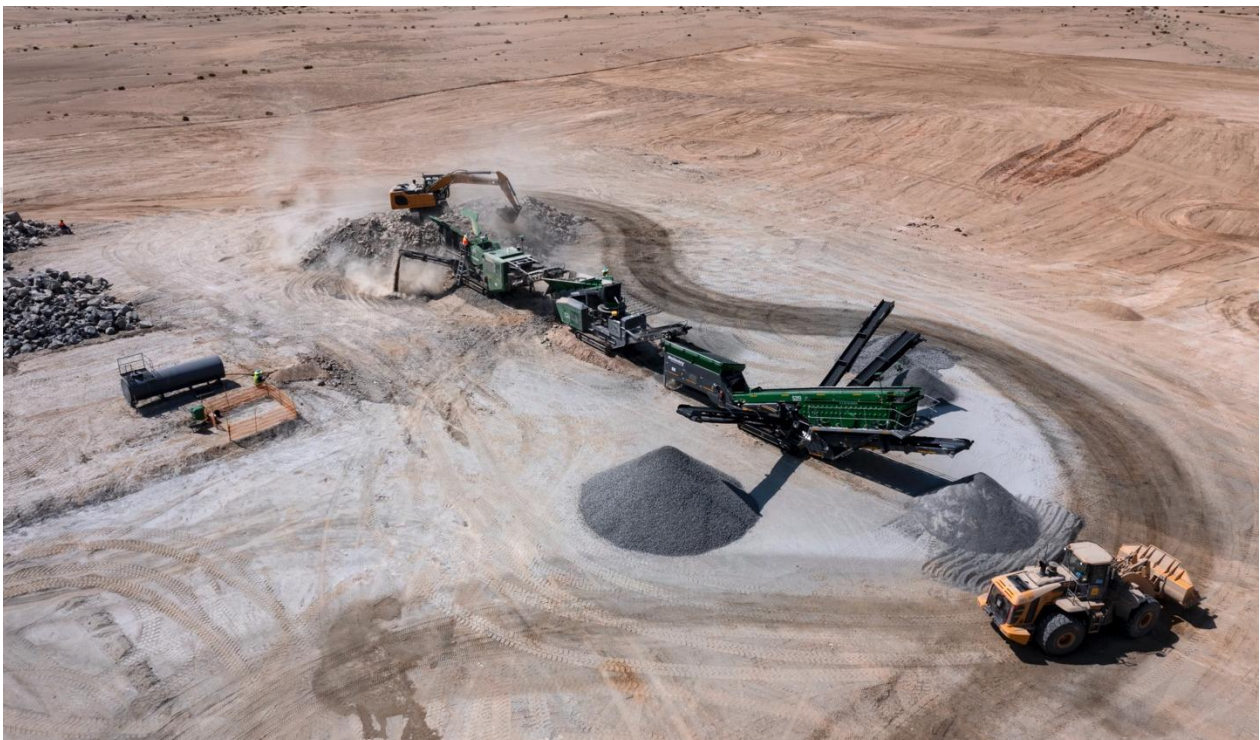
Figure 3: Blasting, crushing and screening of the heap leach drainage material.
