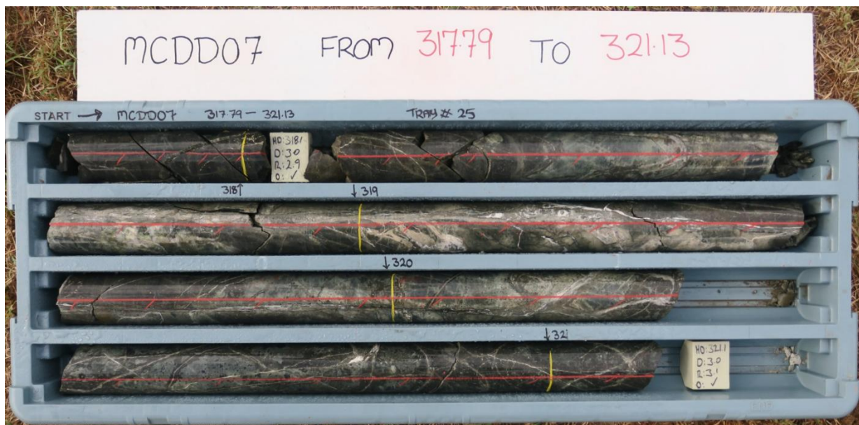
Figure 8: Core tray from MCDD07 showing drilled interval 317.79 to 321.13m. The core shows intense quartz-carbonate veining with pyrite indicative of porphyry-related alteration. Selected intervals will be sampled for assay.
