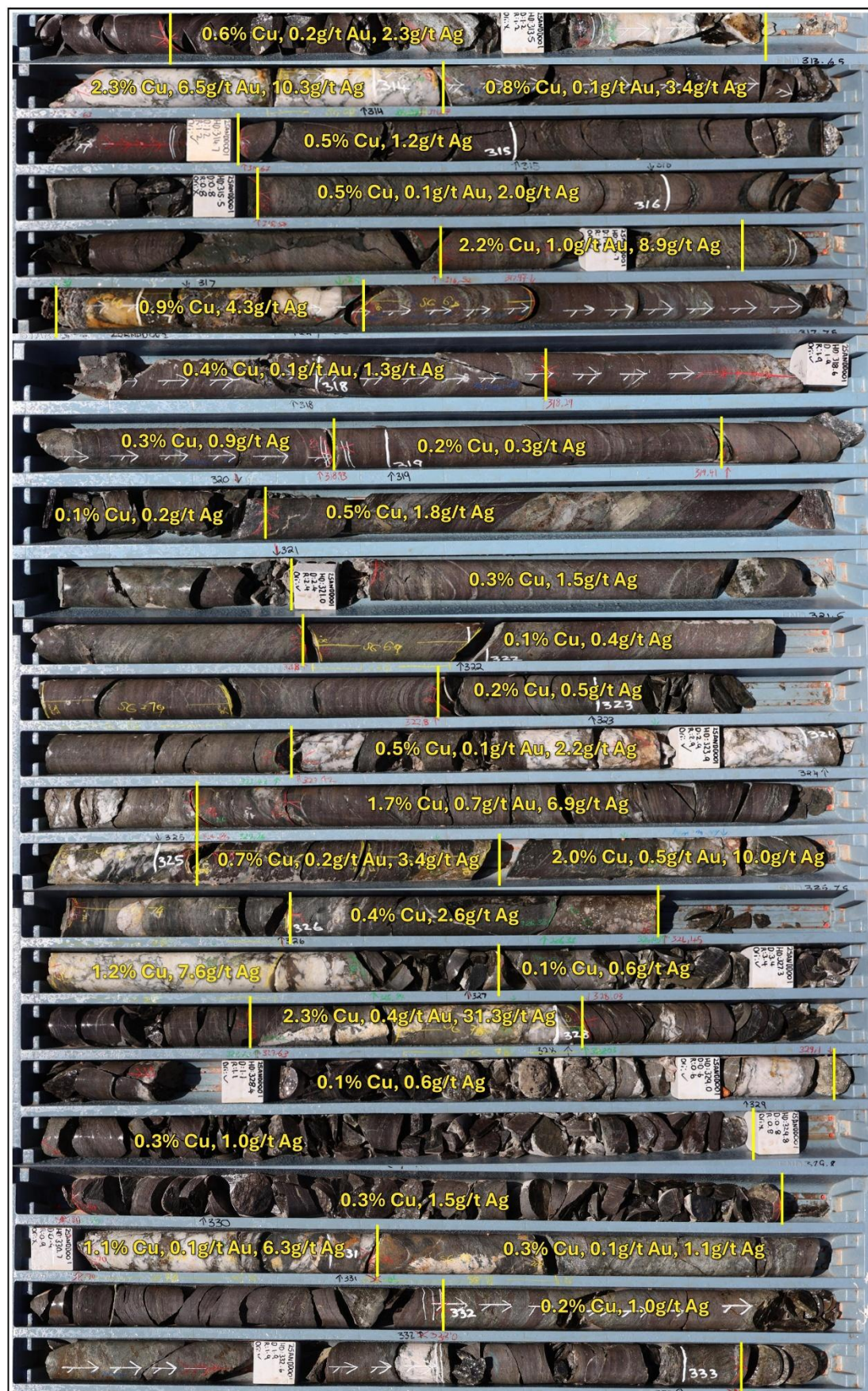
Figure 8: Diamond Drill Core Photos from 313.1 to 333.1 metres in 25ANDD001
