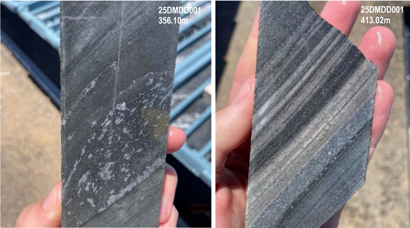
Figure 3: Diamond drill core (NQ size) from 25DMDD001 showing classic BHT (stratabound) lead dominant sulphide mineralisation
