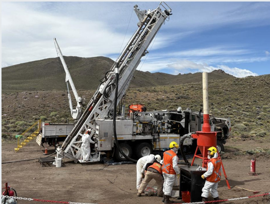
Figure 1: Reverse circulation drilling underway at the Cerro Chacón Gold–Silver Project, Chubut Province, Argentina (December 2025).
