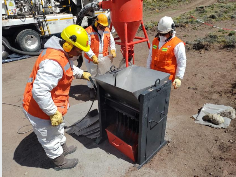
Figure 2: Sample collection during RC drilling at the Cerro Chacón Gold–Silver Project.
