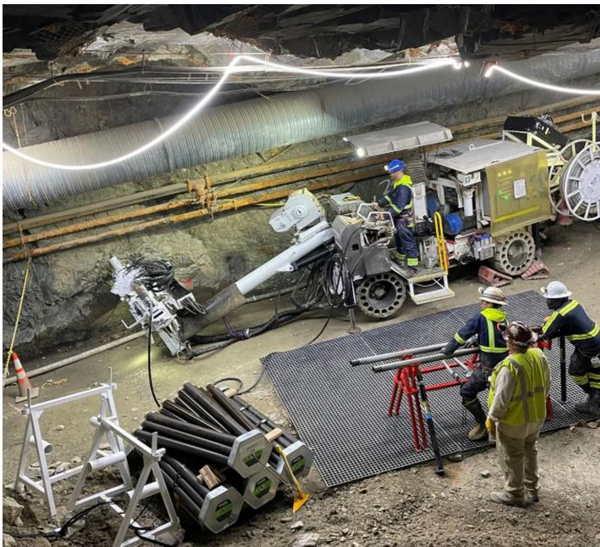
Figure 11: Swick Gen II underground diamond drill rig, drilling DDH251 at crosscut 3 (XC3). 11
