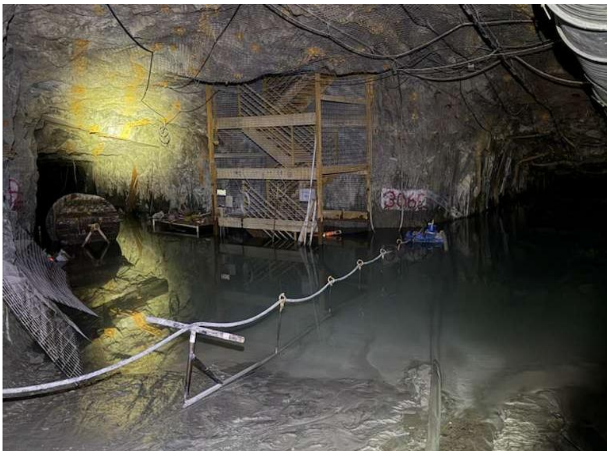
Figure 7: XC5 viewed looking east, picture dated 18 January 2026 Pacific Standard Time (PST). Pump (blue) is shown draining the remaining water from the crosscut. Stairs up to 1030 development drive in mid-shot 14 .
