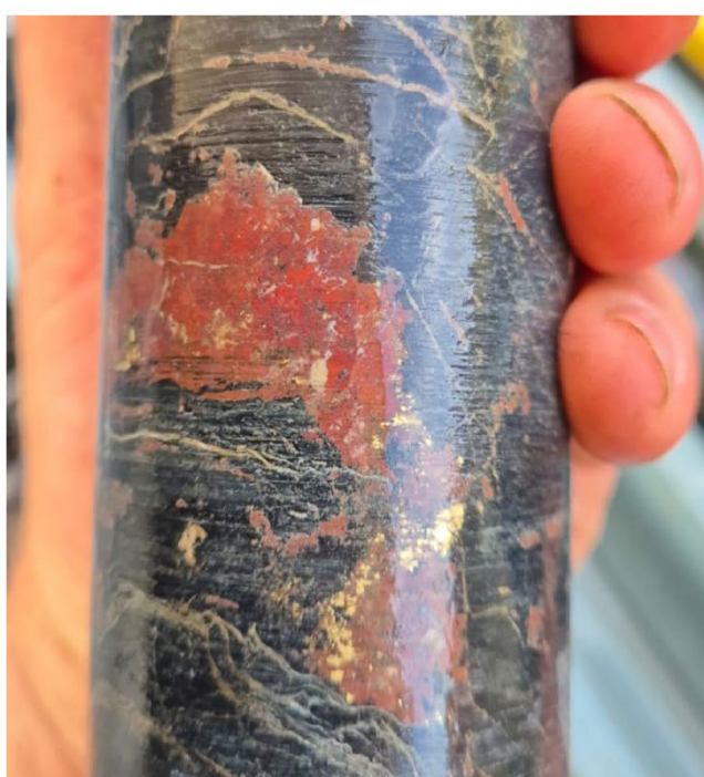
Plate 2 - SDH25-028, 305 meters down hole, visible gold
