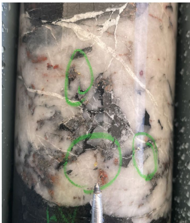
Plate 4 - SDH25-032, 242 meters down hole, visible gold
