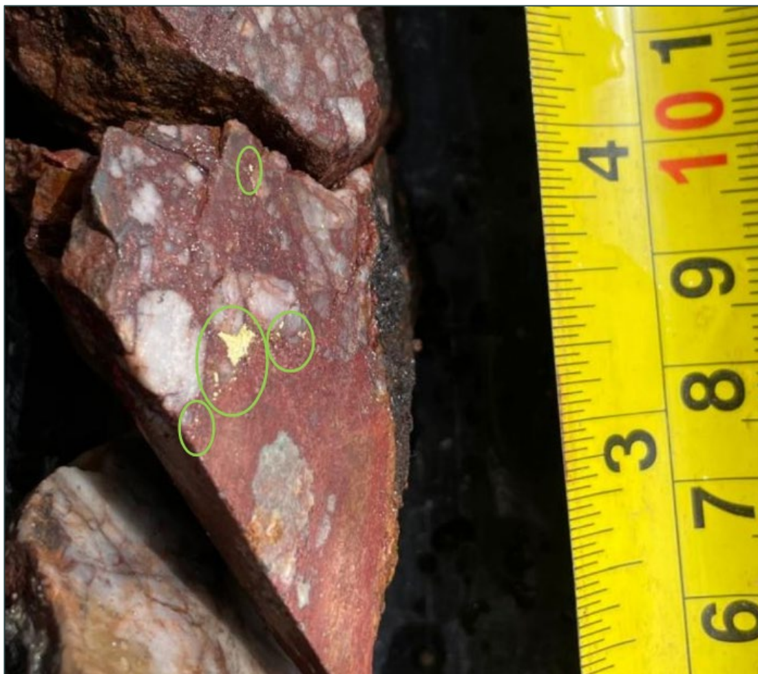
Figure 3 - Visible Gold in oxidised brecciated quartz vein, intersected at 89.47m down hole in SDH25-009
