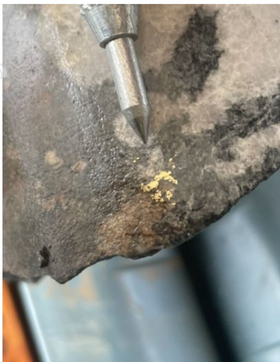
Plate 3 - SDH25-030, 329.2 meters down hole, visible gold
