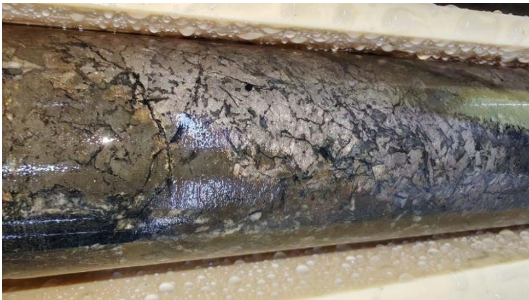
Figure 19: Brecciated semi-massive pyrite (AM25DD001 at 95.7m)
