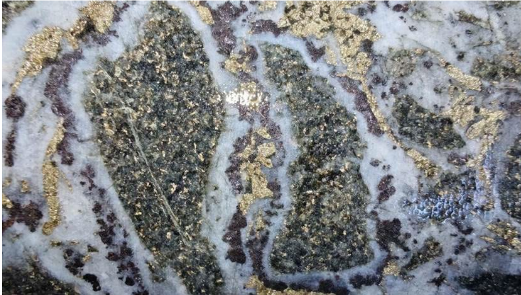
Figure 20: Brecciated and colloform pyrite (AM25DD001 from 95.5m)
