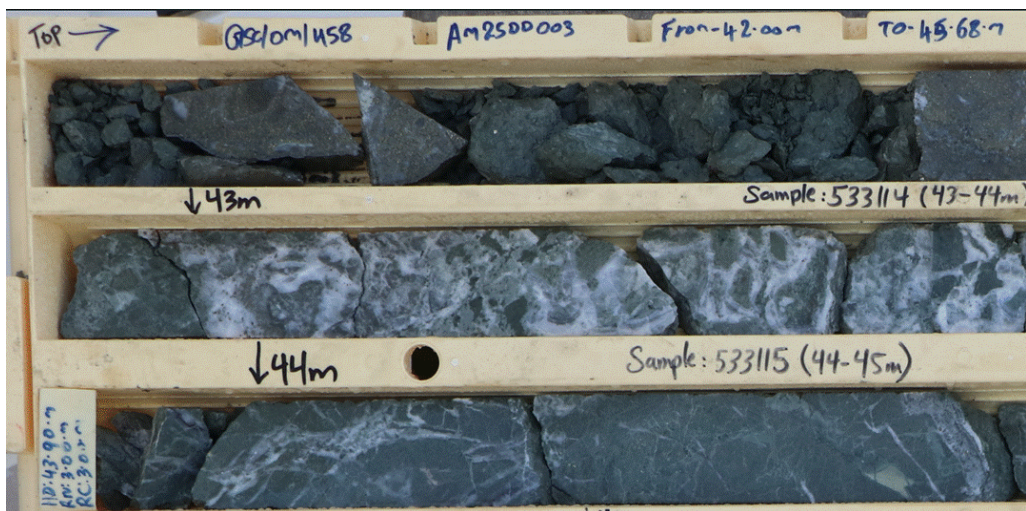
Figure 21: Semi-massive pyrite and quartz breccia/stockworks (AM25DD003)
