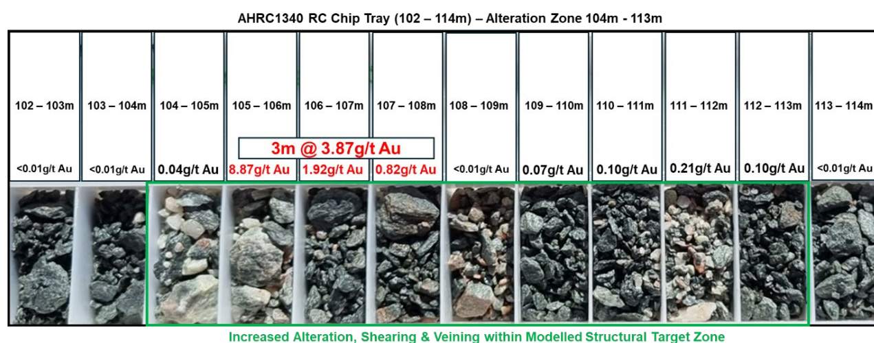
Plate 4 – AHAC1340 RC chip tray images demonstrating alteration, shearing and veining, with a 3-metre intercept at 3.87g/t Au, along with individual metre grades in g/t Au.
