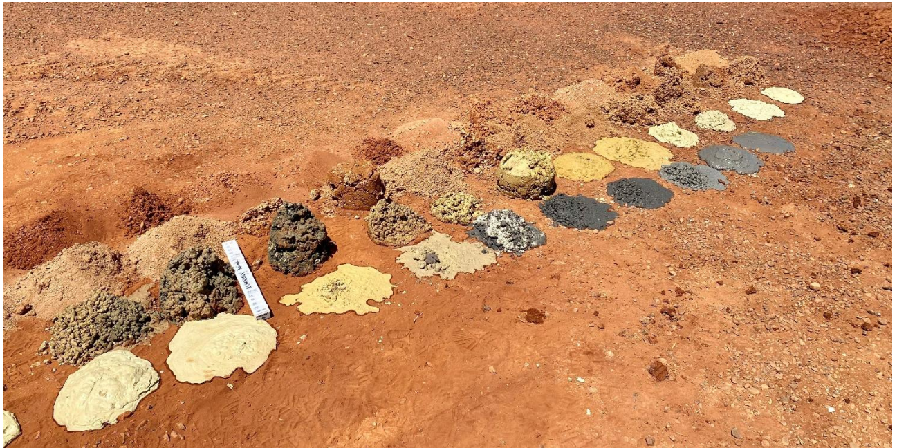
Figure 4. Discovery hole 25YRAC069 (photo taken whilst drilling was still underway at 78m; EOH at 96m). The chip tray marks the middle point in every row of 20 cuttings samples. Note the bright yellow sands associated with mineralisation at 54-56m and 68-72m, overlying black carbonaceous clays at 72-75m and carbonaceous sands from 75m onwards.
