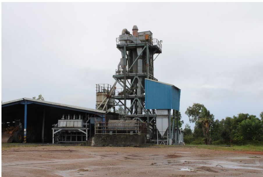
Figure 6 Graphite concentrate dryer at Graphmada
