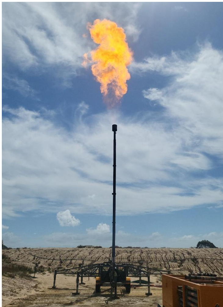
Figure 4: Wombat-5 gas flare on 19 January 2026, following blowing down with Nitrogen
