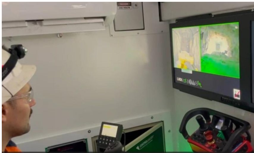
Image 5: Tele-remote bogging in 1438 North stop
