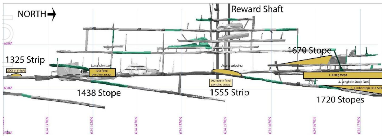
Image 3: Longitudinal section of the Reward underground workings showing the Lady Belmore Reef adjoining (including the 1438 Stope)
