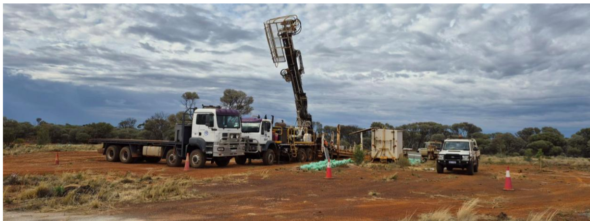
Figure 1: Diamond drilling James Stage 1 metallurgical testwork hole
