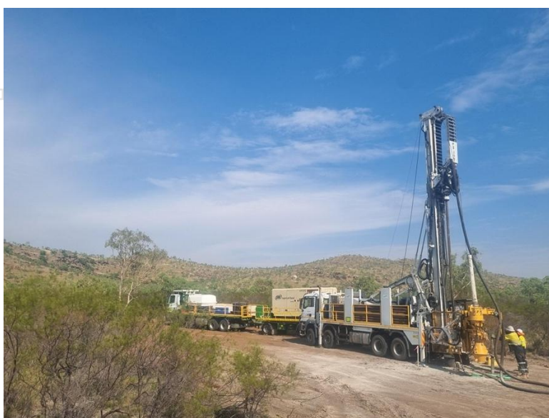
Figure 11: RC drill rig set up on Hole 24RCDH03
