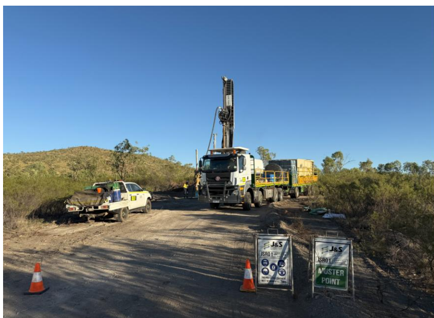
Figure 10: RC drill rig set up on Hole 24RCDH02
