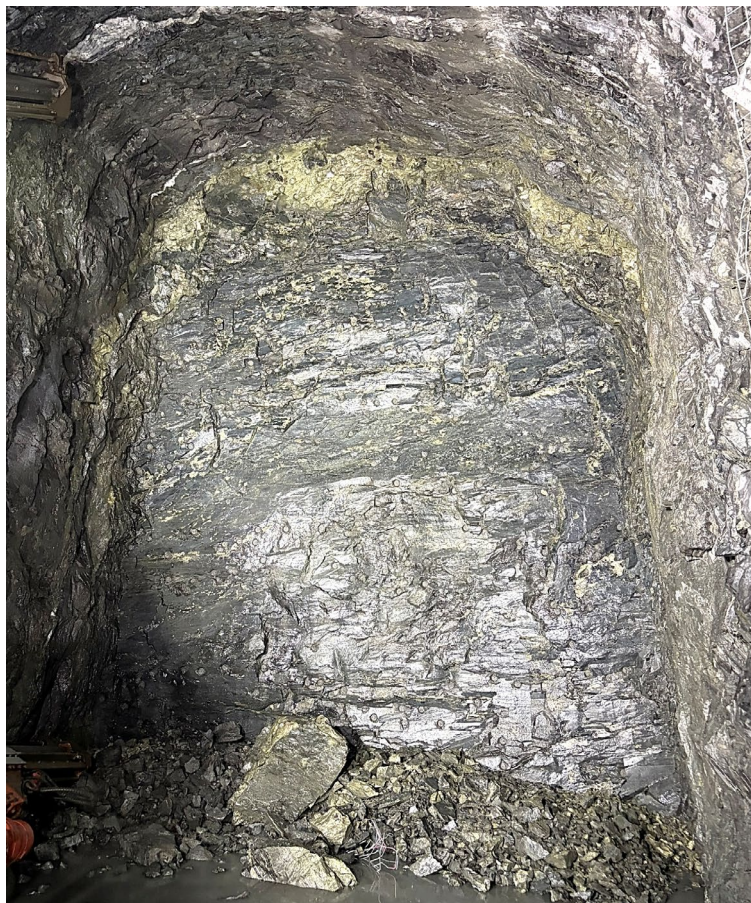
Photo 1. Development face passing through the J1 lens at Jericho, showing visible copper sulphide mineralisation. Face dimensions are approximately 5.5m wide by 7.5m high.
