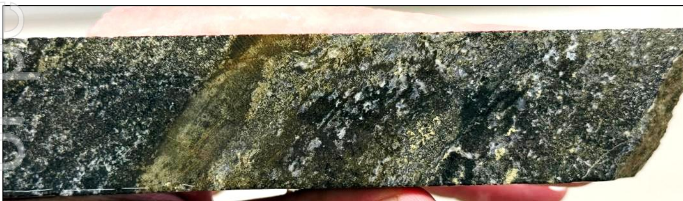
Figure 6. Core photograph from 348.4m to 349.6m in ZRSD25221, showing green garnet skarn with disseminated to semi-massive pyrite-chalcopyrite-sphalerite-galena – 6.7g/t Au, 0.2% Cu, 0.6%Pb, 0.9% Zn, 37.6 g/t Ag (8.3 g/t AuEq 2 ).
