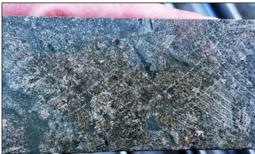
Figure 8. Core photograph from 616.0m to 618.0m in ZRSD25232 showing green garnet skarn with disseminated to semi-massive pyrite-chalcopyrite-arsenopyrite – 7.3g/t Au.
