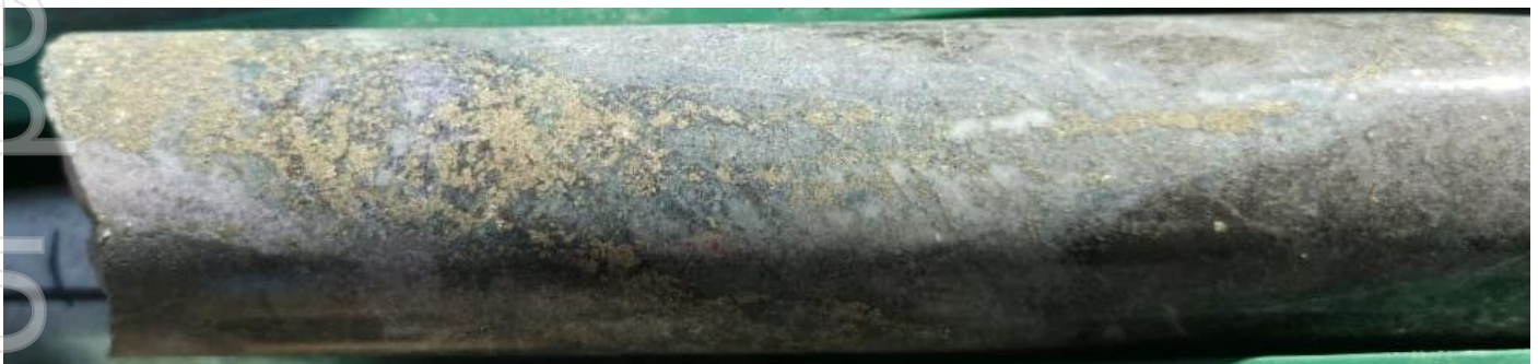
Photo 2. Pyrite-Chalcopyrite disseminated sulphide from 1,359m downhole in 25LHDD071* (refer to Appendix 1).
