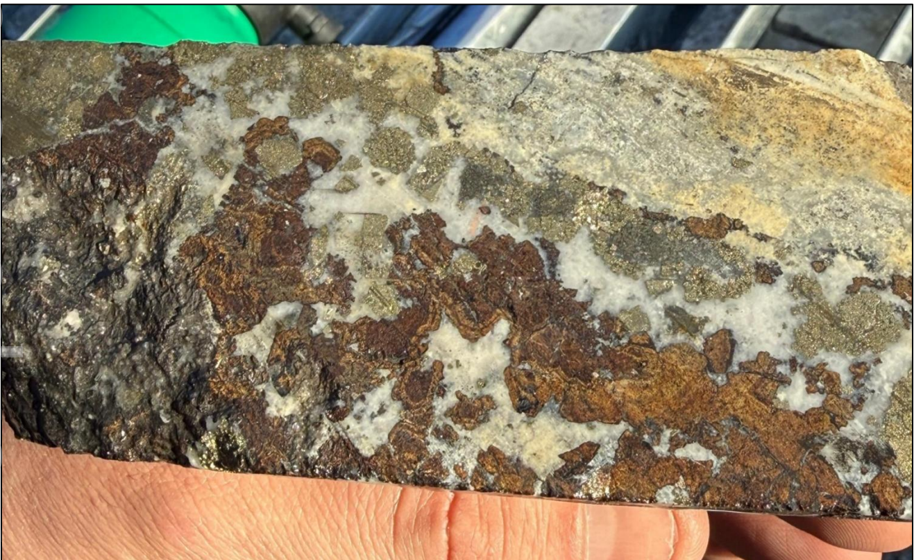
Figure 6: Core photograph of semi-massive sphalerite with disseminated pyrite, galena, chalcopyrite and carbonate veining from the interval of 538.5 to 540.5m – 0.6g/t Au, 0.3% Cu, 1.1% Pb, 7.9% Zn and 13.6g/t Ag (6.0g/t AuEq 2 ).
