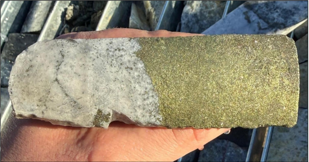
Figure 5: Core photograph of massive chalcopyrite with carbonate vein from the interval of 524.5 to 526.5m – 0.4g/t Au, 1.4% Cu, 0.2% Pb, 0.1% Zn and 15.5g/t Ag (3.3g/t AuEq 2 ).
