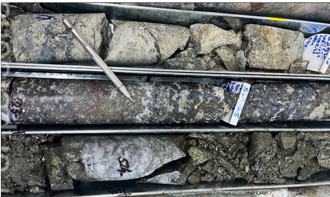
Figure 1: Core photograph of semi-massive to massive sphalerite, galena, pyrite and chalcopyrite with carbonate veining from 522.0m to 524.5m down-hole in ZRSD25233 – 2.8g/t Au, 3.7% Cu, 5.3% Pb, 1.5% Zn and 86.6g/t Ag (13.5g/t AuEq 2 ).
