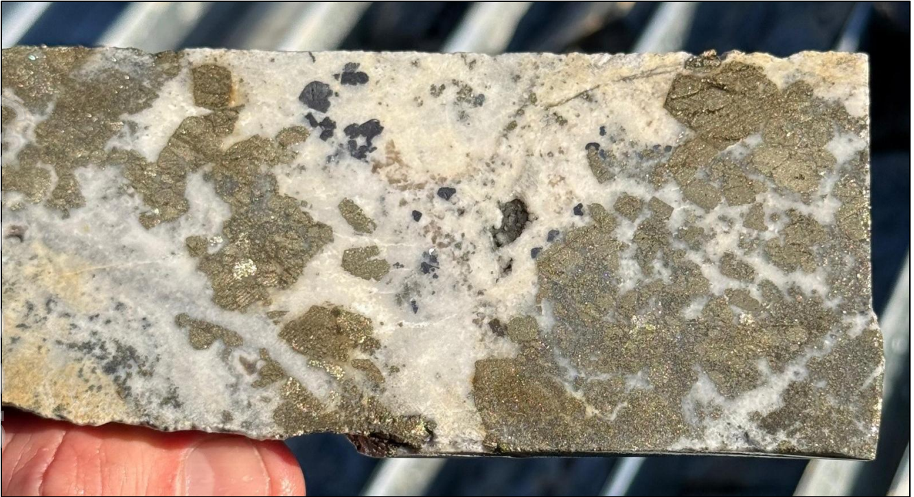
Figure 7: Core photograph of carbonate veining with disseminated to semi-massive pyrite, galena, chalcopyrite and sphalerite from the interval of 540.5 to 542.5m – 1.9g/t Au, 0.3% Cu, 1.1% Pb, 0.8% Zn and 17.3g/t Ag (3.6g/t AuEq 2 ).
