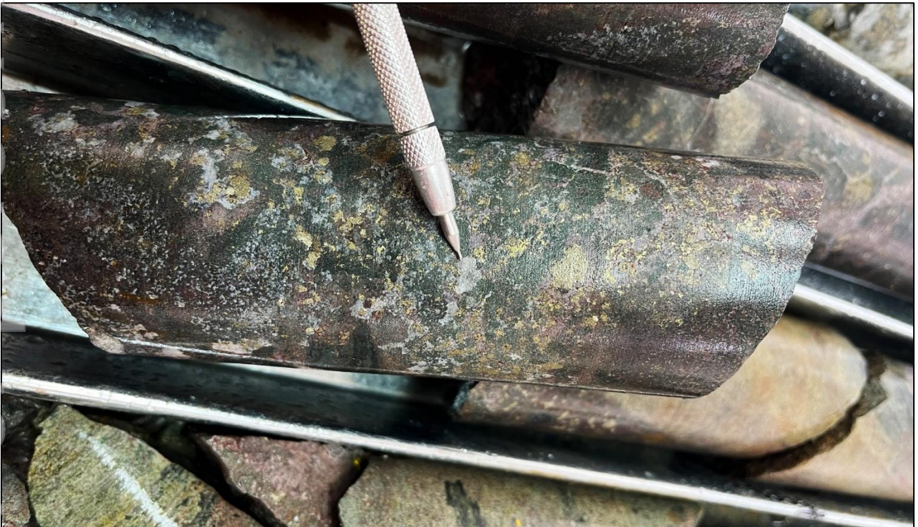
Figure 8: Core photograph of disseminated pyrite and chalcopyrite with magnetite alteration from the interval of 551.4m to 553.4m – 1.2g/t Au, 0.6% Cu and 4.3g/t Ag (2.3g/t AuEq 2 ).
