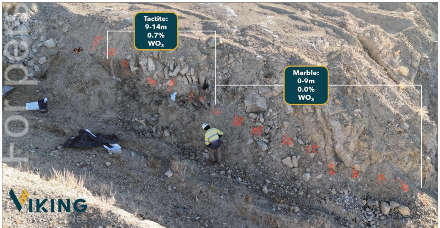
Figure 4; Photo showing LKCH0001 channel sample at Linka Pit with outcropping mineralised intervals of 5m at 0.7% WO_3 .
