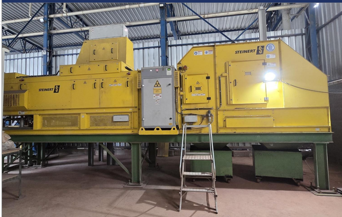
Steinert KSS CLI XT combination sorting system incorporating X-ray transmission (XRT), 3D laser and inductive sensors
