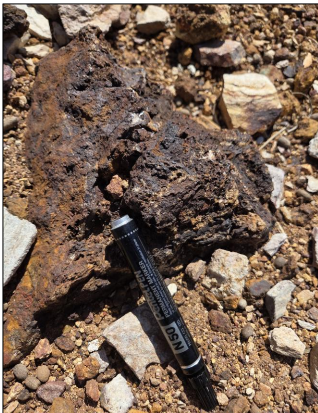
Figure 2: Gossanous material adjacent to Wednesday Shaft – with sample MP20250903-1 assaying 3.10% Sn , 3.03% Pb, 0.33% Cu, 0.27 Zn & 158.5ppm In.
