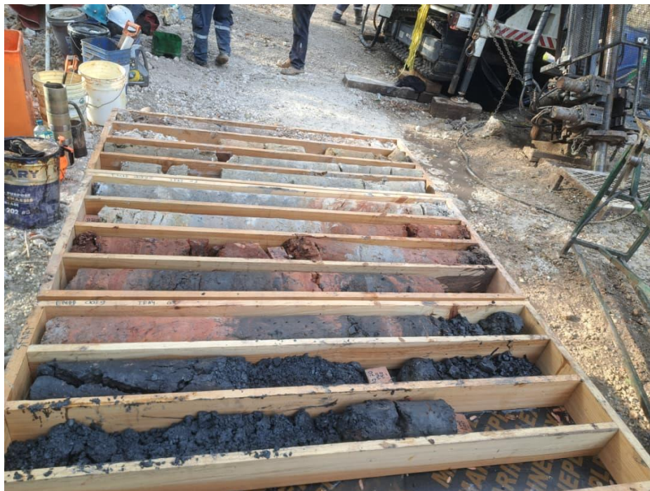
Figure 4: Manganese bearing red clay overlying main mineralised zone in EMDD039 2
