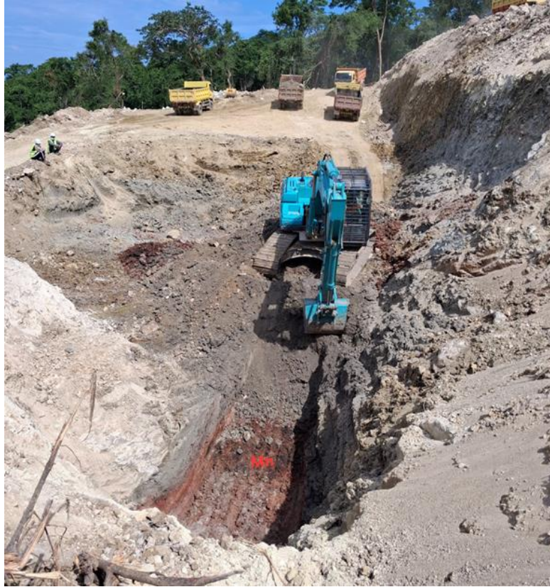
Figure 3: Exposure of manganese bearing red clay interpreted to overlie main mineralised zone (see Figure 4) within excavation 2
