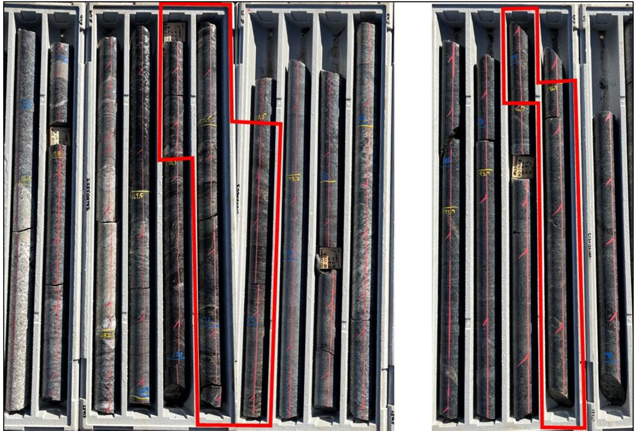
Figure 2. Sulphide rich zones in BDCDD2503 at 170.5m-172.5m downhole and 194.9m-195.9m downhole 2
