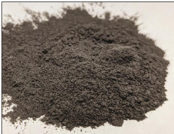
Figure 3: Antimony sulphide (37% Sb) precipitated from leach liquor
