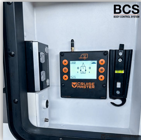
The heart of Cruisemaster BCS, user interface for control of air suspension and tyre inflation.
