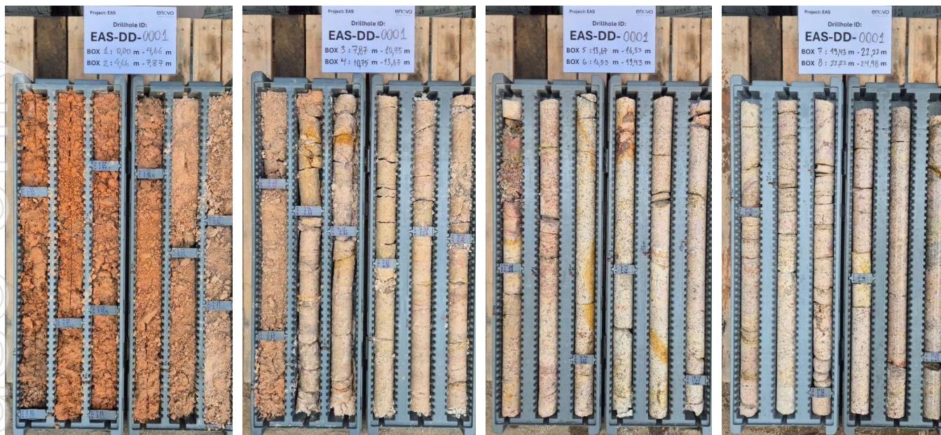
Figure 6: Saprolite clay in EAS-DD-0001 diamond hole
