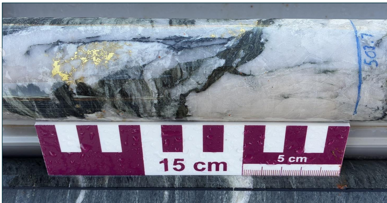
FIGURE 3: COARSE GOLD FROM 503.52 TO 503.77M IN 25MBRCD002A
