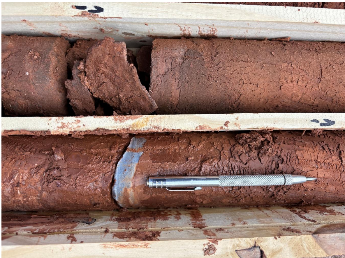
Figure 2. The claystone unit showing a large anhydrite secondary filling in the fracture. The unit is entirely non-porous clay.
