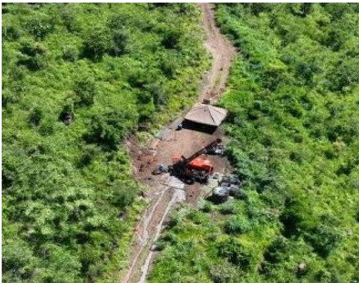
Figure 1: Diamond core drilling underway at Kangankunde. Aerial view of the drill pad supporting the Stage 2 resource definition program targeting Inferred-to-Indicated conversion areas.
