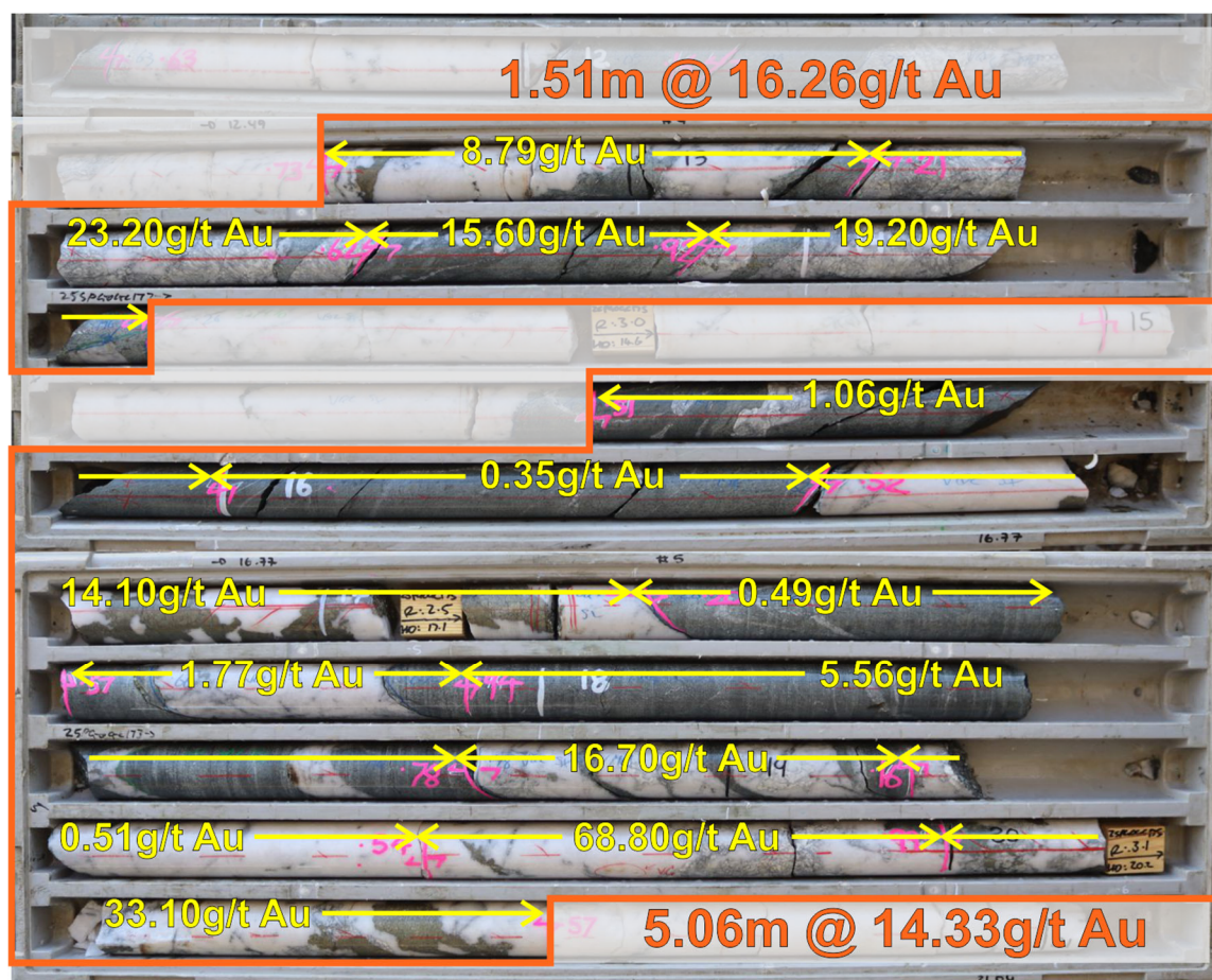
Figure 1: Core Photo of 25PGOGC175 showing two intercepts – 1.51m @ 16.26g/t Au from 12.73m and 5.06m @ 14.33g/t Au from 15.51m.
