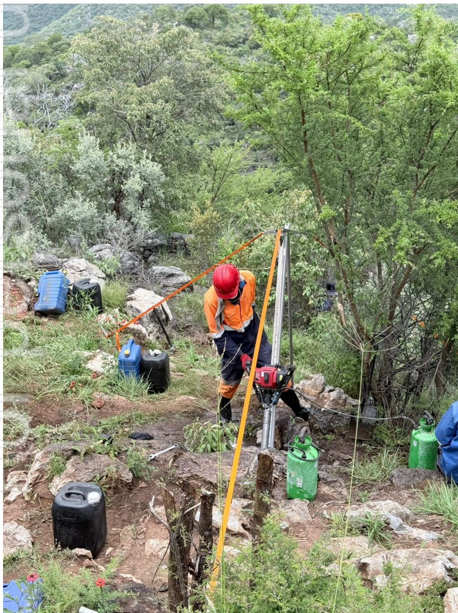
Image 1: Graceland Prospect. Lightweight diamond drilling rig testing Gossan 1 East mineralised zone - with new frame.
