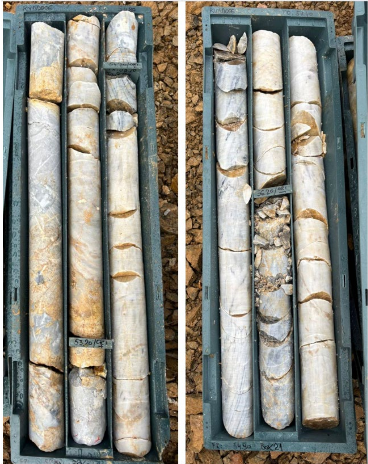
Figure 2: Unprocessed PQ drillcore from hole KVDD006 (note: hole numbering is not sequential), showing brecciated marbly limestone and barite at the target depth, from ~52m to ~57m, and with sporadic galena-sphalerite mineralisation.
