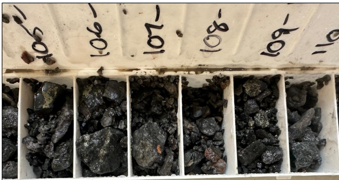
Figure 3. Logged sulphides and quartz veining CWRC25-43. Maximum 1m assays; gold 0.02 g/t Au, arsenic 31 ppm and copper 431 ppm.
