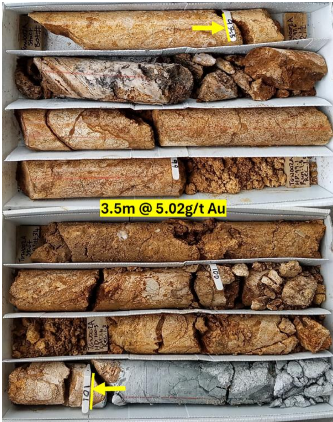
Figure 3: TGW002A core tray photo, high-grade zone 3.5m @5.02g/t Au, 97.5m – 101.0m
