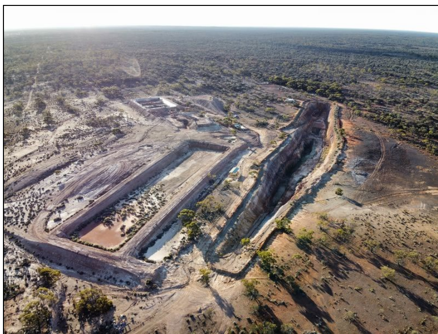
Figure 4: Drone photo of Zelica Project looking NNW showing pre-stripped open pit (approx. 300-400m long and 10-25m deep) and pre-constructed vat leach ponds (pic taken August 2025)
