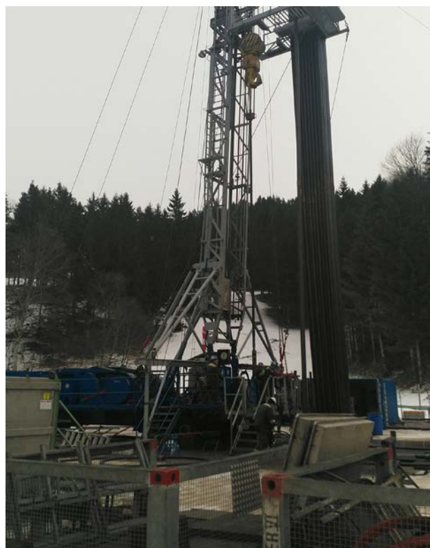
Figure 2: MB Well Services AW-24 rig running tubing at Welchau-1 well in preparation for testing
