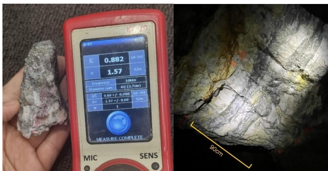
Figure 3: Left: Very high-grade grab sample (358.0g/t Au & 1,800g/t Ag) showing typical magnetic susceptibility & conductivity readings. Right: Banded sulphides in the backs of the South Black Bear Vein.
