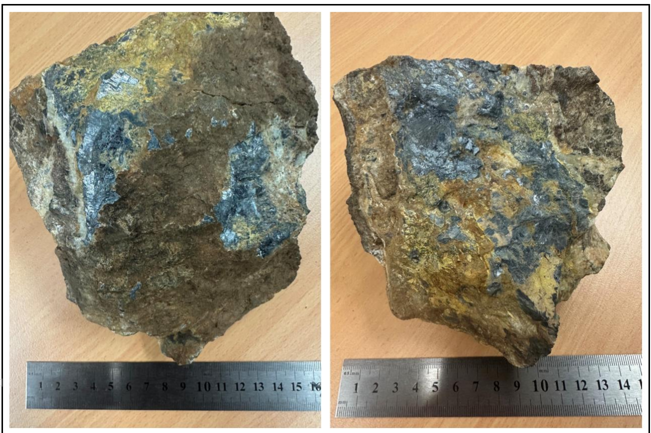
Figure 1: Examples of-mineralised material collected and submitted for metallurgical testing, with coarse grained silver stibnite crystals..
