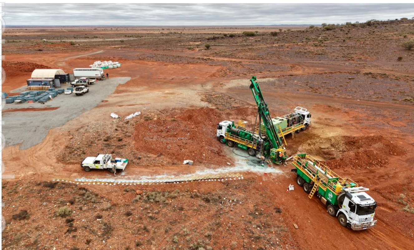
Figure 1: Hagstrom, Schramm T685 heavy duty RC rig and booster completing first pre-collar to depth.
