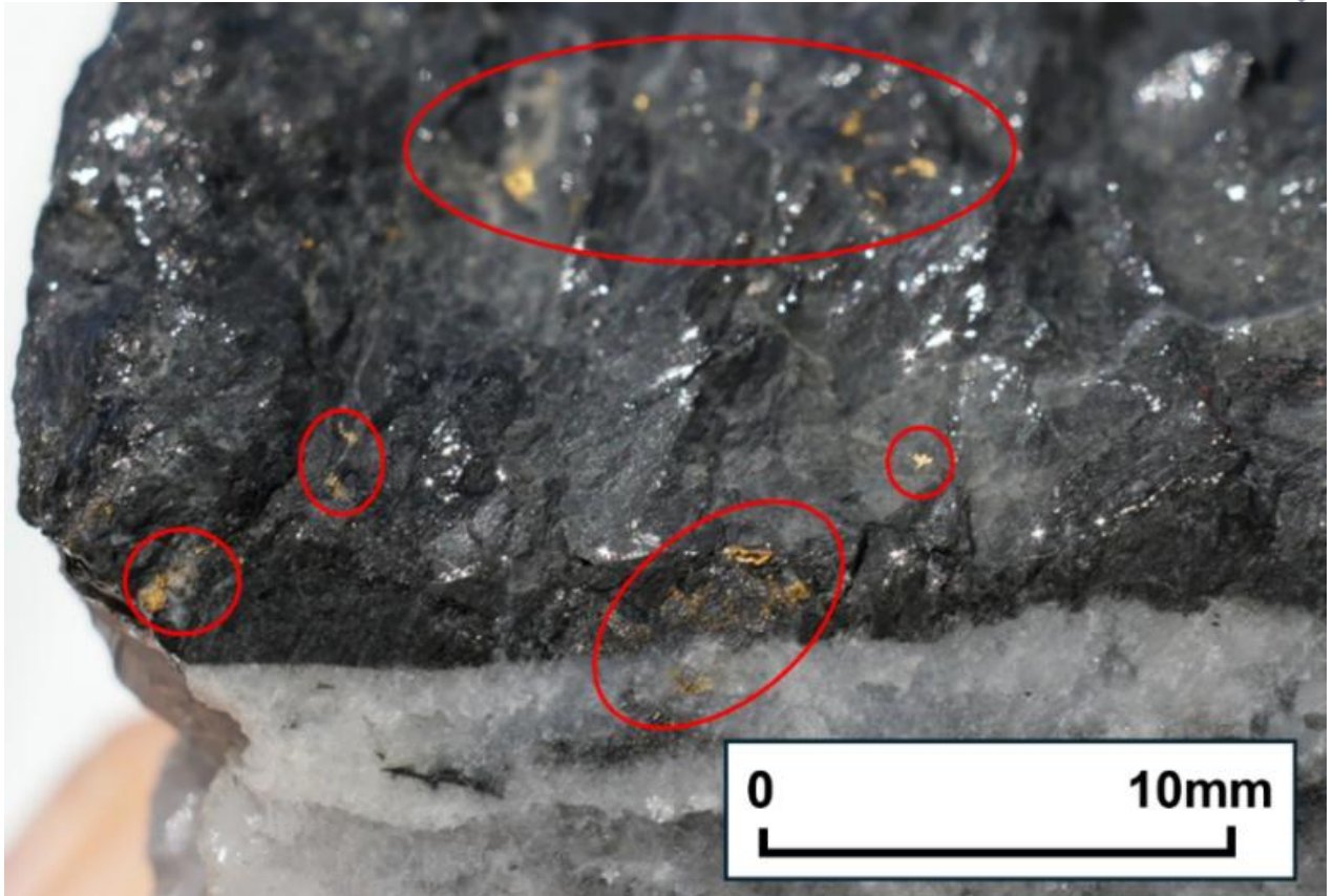
Figure 2 BMDD004W1 showing visible gold (red circle) in a quartz carbonate vein at 635.4m (downhole depth)
