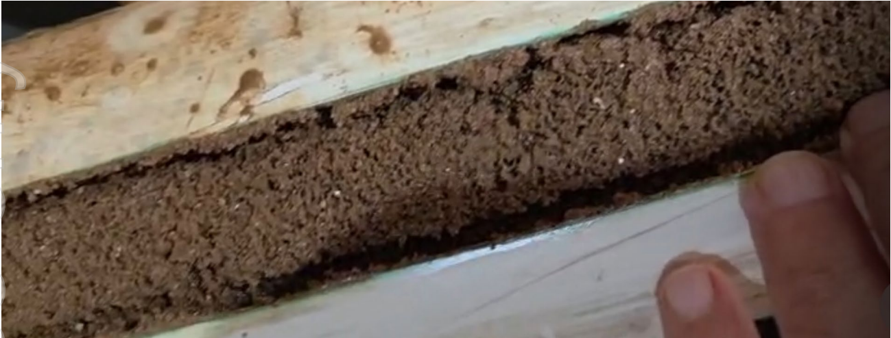
Figure 4 – 90% Rougher spirals tails + 10% thickened slimes after natural free draining test
