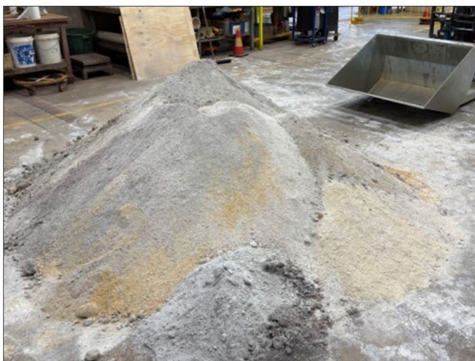
Figure 4: Three tonne bulk sample (RM04), averaging 13.0%HM, undergoing preparation for spiral separation
